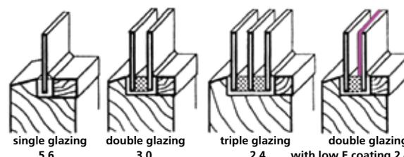
Figure 16: U-value against cavity width for glazing (unit: W/m<sup>2</sup>K)
