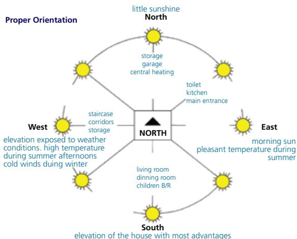
Figure 12: Proper orientation of a building (north hemisphere)
