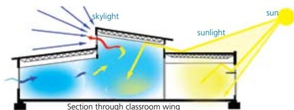
Figure 5: Daylighting concept
