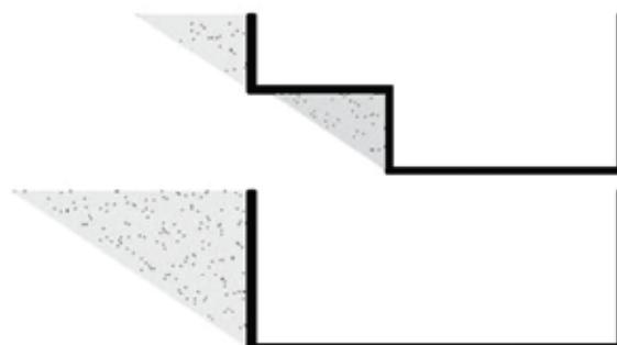
Figure 15: Effect of plan on self-shadowing
