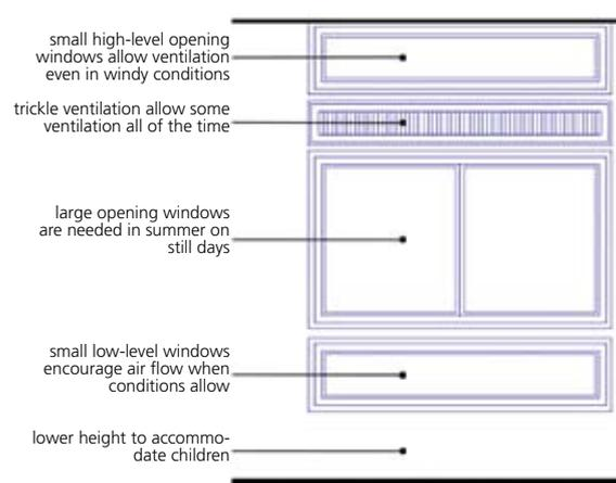
**Figure 18:** Ventilation options for varying conditions
