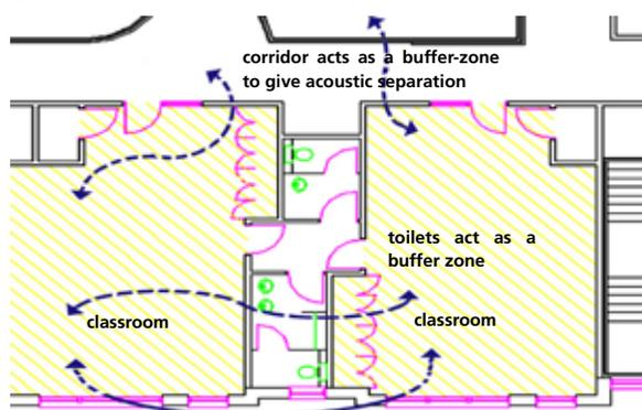
Figure 9: Use the toilet and corridor as buffers from the noise (Confirmatory Case)
