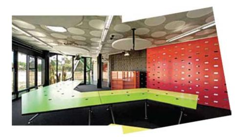
A futuristic workshop space. The circular drop down ceiling panels form part of the ventilation, heating and cooling system. (This photograph is used with the permission of Lyons-Architects. Photograph credit: Gollings Photography)
